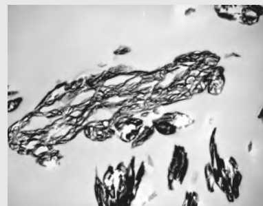
TEM CROSS-SECTION OF OPACILITE™
