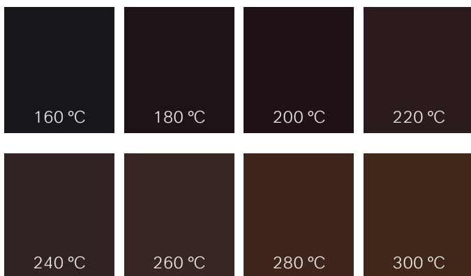
Figure 7: Color change of an iron oxide black pigment (magnetite) in a coating system based on phenylmethylpolysiloxane
