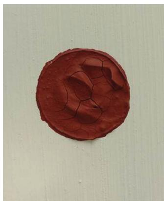
Panel contaminated with iron oxide dirt
