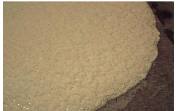
No bleeding with addition of 0.8% Cembinder 50 bwoc
